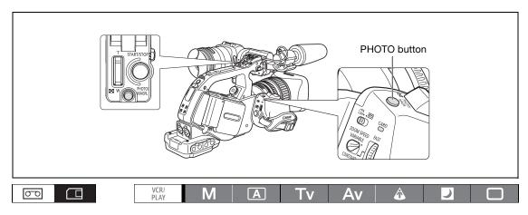
1. Turn the POWER dial to a recording program and set the □/ □ (card/tape) switch to □.
